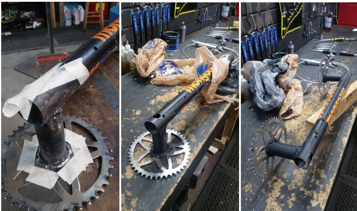
The weld areas were cleaned of slag then masked around the welded/burned areas then primed and painted black to prevent rust
