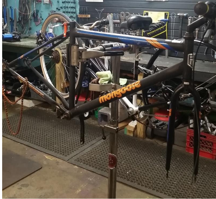
Scrap bike frame selected as tubing donor for the tool rack
