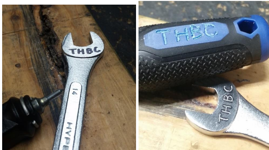
The tools were engraved with our Co-op initials to discourage theft. The engraver tool is a common carbide point electric reciprocating engraver tool (not a rotary tool).
