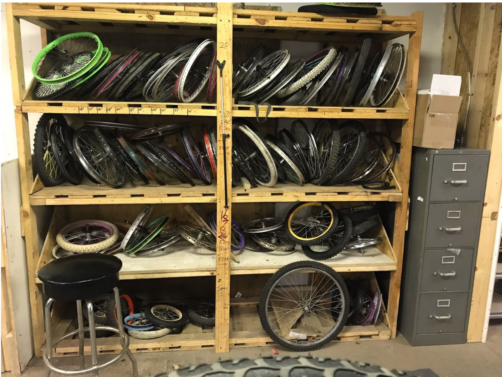
We store 20" and smaller rims on a rack made from surplus shipping pallets and 2x4s.
